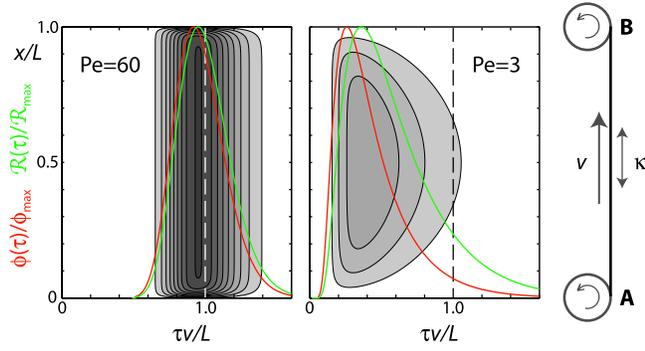
**Figure 1.** Shading: Contour plot of  $\eta(x, \tau)$  for the idealized conveyor model of the schematic to the right. The contour interval is  $0.25 v/L^2$ . The curves  $\mathcal{R}(\tau)$  (green) and  $\phi(\tau)$  (red) have been normalized by their peak values and superimposed.
